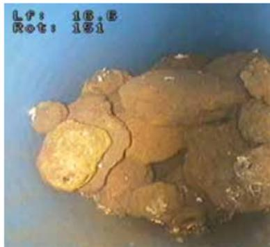
Problems found included broken casings, obstructed pipes, and defective pumps, but also contamination of the water. At one borehole, the potentially harmful fluoride content of the water was reduced by sealing a section of the borehole at 46 meter depth.
