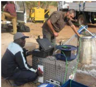
The project equipped a vehicle with a submersible camera, a data logging probe, a spectrometer, a compressor, pumps and brushes. With this mobile workshop and the help of local workers, 50 boreholes were diagnosed between 2013 and 2015 – and 31 (62%) were rehabilitated.
